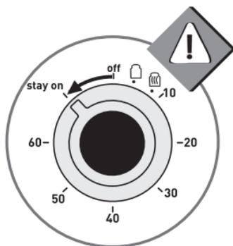
Set the timer dial on « Stay on ». The power indicator light turns on and keep warm starts.
