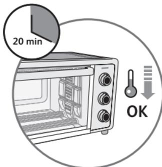
Disconnect the appliance and let it cool down completely before cleaning or storing.
