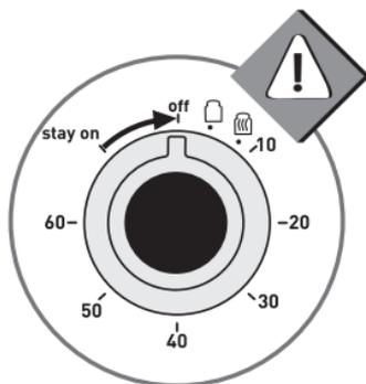
To stop the keep warm function, turn the timer button to « off » position; the indicator light will turn off.
