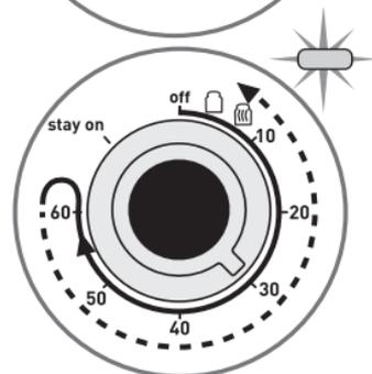
Turn the timer to the desired setting. The power indicator light turns on and cooking starts.
