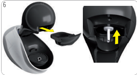
6 Remove capsule holder. Push injector tool over injector.
