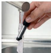
You can remove the steam nozzle for thorough cleaning. Wash it using a brush with water and a little non-abrasive washing up liquid. Rinse and dry it. Before re-fitting, make certain that the air inlet holes are not clogged by milk residues. Clean out the holes with a needle if necessary.
