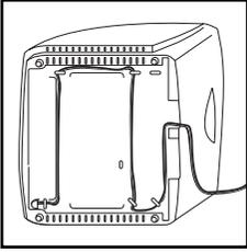
Never wrap the cord around the outside of the appliance during or after use. A cord storage is located under the appliance.
