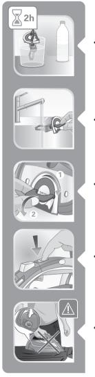
• To descale the Micro Calc filter thoroughly rinse it in diluted citric acid for 2 hours.
