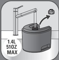
**EN** Remove the cap, fill in the water tank, then fully screw the water tank cap.
