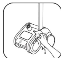
**TIP:** For more effective descaling, after every 50 hours of use, use descalers available at your store recommended for garment steamers or electric kettles. To avoid irritant vapors, use products based on citric acid only.
