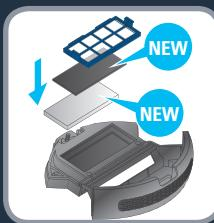
**EN** Every 6 months replace the fine dust and foam filter with new ones to maintain optimal performance.
