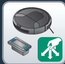
**EN** Attention: Before removing the battery turn off the robot. Turn the robot upside down to get access to the battery slot. Remove the battery by pressing snap latches of the battery slot and pull the battery up. Disconnect the battery from the robot. Recycle the battery and robot.
