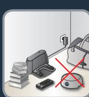
**EN** To place the docking station, make sure there is an empty area of 1m on each side and 2m in front of the docking station. Do not install the docking station near stairs. The cable must be tight. Always place the docking station on hard floor. Do not place the docking station on carpet.
