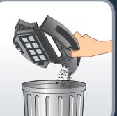
**EN** The robot should be emptied and cleaned at least once a week. Push the button on the backside of the robot and pull out the dust container. To empty it, flip off the cover.
