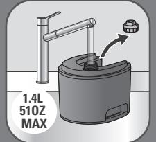
**EN** Remove the cap then fill in the water tank until maxi-mark, fully screw the water tank cap.
