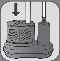
**EN** Insert the first segment in the housing and screw in fully by hand.
