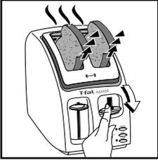
Push down the hi-lift lever (right lever).
