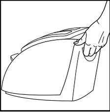
To move the toaster, a carrying handle is located at the back of the appliance.
