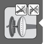
The fabric brush opens the weaves of the fabrics for better steam penetration. Attach the fabric brush to the steam head when appliance is unplugged.
