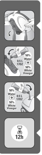
Vertically tilt the appliance to empty water in a sink.
