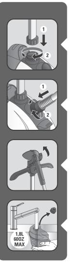
Insert the pole in the housing & then screw until lock.
