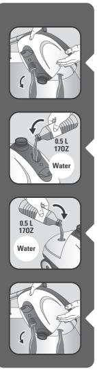
Vertically tilt the appliance to empty mix in a sink.
