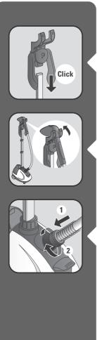
Fully insert the hanger vertically on top of the pole.
