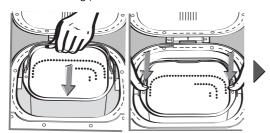
Place the bread pan in the breadmaker. Replace the bread pan and press on one side then the other to engage the mixer drives and clip it in on both sides.
