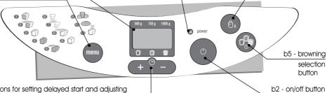
b4 - buttons for setting delayed start and adjusting
