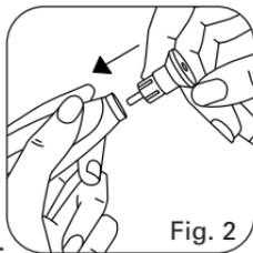
**Attention!** Always unplug the device when mounting accessories and clip them firmly into the housing (push the accessory until you feel resistance Fig.2).
