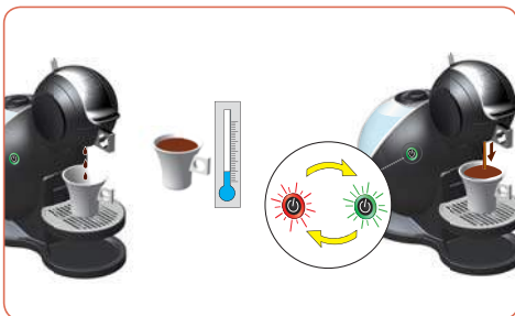
If the beverage only comes out in droplets or if the beverage is cooler than usual, the machine has to be descaled.
