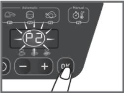
11 The selected program stays displayed at the top of the screen.. Press the “-” and “+” buttons to select the desired cooking level (rare, medium, well done). Once you have reached the desired cooking level, press the 'OK/START' button. The selected cooking stays displayed at the bottom of the screen.
