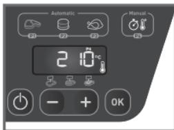
24 Press the “-” and “+” buttons to select program P4. When the P4 program is reached, press the “OK / START” button.
