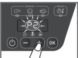
10 Press ON/OFF. Press the “-” and “+” buttons until you reach the desired program (P1, P2, P3).
