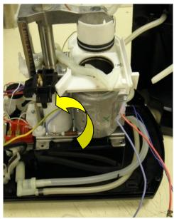
Unscrew the two (2) switch screws
