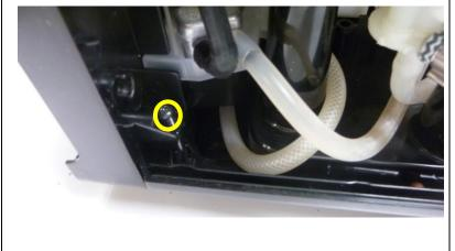
Open the front panel by lifting the grinder plate and disconnecting the coffee line.
