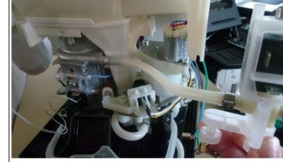
Turn the solenoid valve to position it on the base and create the loop on the line (to prevent kinks).
