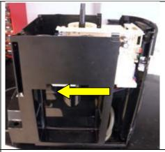
Disconnect all the wires from the board
