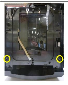
Remove the two (2) screws at the back
