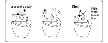
from main unit by releasing container lock and pulling up. Unscrew the cover and fill. Do not fill above the max line on the water tank. Water container capacity is 3.4 quarts.
