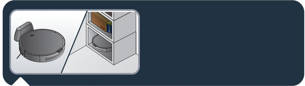
**EN** In order to extend the battery lifespan, always keep the robot charging on the docking station while not using it. If the robot is stored off/out of the docking station, make sure the robot is OFF and the battery is fully charged. Store the robot in a fresh and dry place. Please charge the robot every 3 months when you are not using it.
