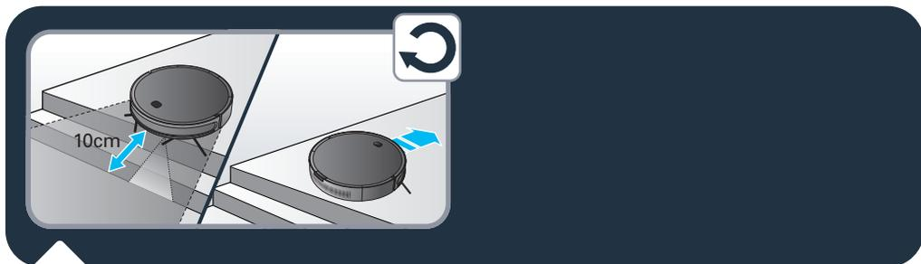
**EN** The robot has drop sensors to detect stairs and gaps. The robot will change direction when detecting them. In order to correctly detect the floor level difference, make sure there are no objects (bags, shoes...) on the floor next to gaps, stairs or on the stairs' steps. The step must be more than 10 cm away to be detected.
