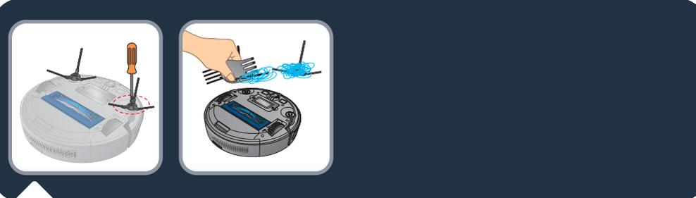
**EN** To clean the side brush, remove it and use a cleaning brush to clean the side brush and the entanglements in the slot of the side brush. Replace lateral brushes every 6 months.
