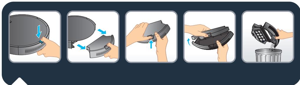
**EN** The robot must be emptied and cleaned after each use. Push the button on the backside of the robot and pull out the dust container. To empty it, flip off the cover.
