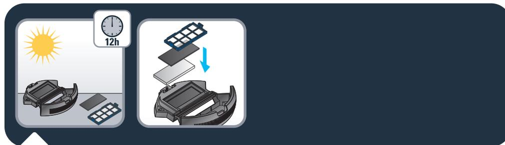
**EN** Let all parts dry approximately 12 hours. Do not use wet filter or dust container. When dry put the filters back in the dust container.
