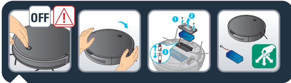
**EN** Attention: Before removing the battery turn off the robot. Turn the robot upside down to get access to the battery slot. Remove the battery by pressing snap latches of the battery slot and pull the battery up. Disconnect the battery from the robot. Recycle the battery and robot.
