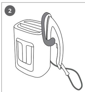
**EN** Position the iron and its iron rest on the steam unit.
