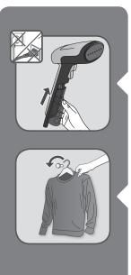
Return the water tank to its place by sliding it up until completely set. Make sure that water tank is fully set in place.
