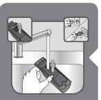
Fill the water tank with 100% water and repeat the operation until the water tank is completely empty in order to rinse the appliance.
