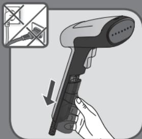
Remove the water tank by sliding it down.
