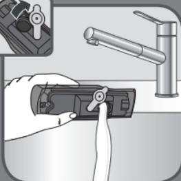
Empty the water tank completely and then close the water inlet cap.
