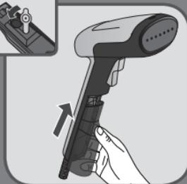
Return the water tank to its place on the appliance. Make sure the water tank is fully set in place.
