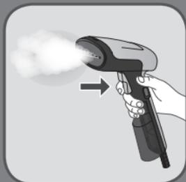
Press the steam button with the steam head facing away from you holding it in a vertical position.
