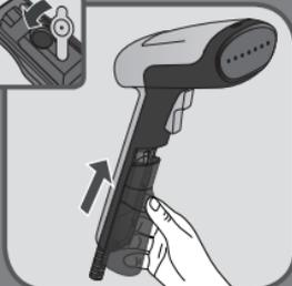
Return the water tank to its place on the appliance, make sure it is completely in place.
