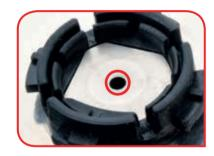
Before reinstalling the ball, check that the pipe is not blocked by blowing into it.
