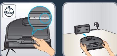
Turn the robot on by pressing and holding the START button until the robot lights turn on (~5 seconds). Manually place the robot against the station. Wait 3-4 hours for the robot to be fully charged. For the first-time cleaning, please ensure that the robot is fully charged. For the first cleaning in a new environment, the robot will create the home map. In order to improve the accuracy of the map, don't use the vibrating water tank, keep the « vacuum only » module installed in the robot.
