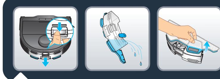
At the end of the cleaning session, unclip the water tank by pressing the latch and pull to remove the water tank. Empty the water tank of the remaining water. Remove the dirty mop cloth.
