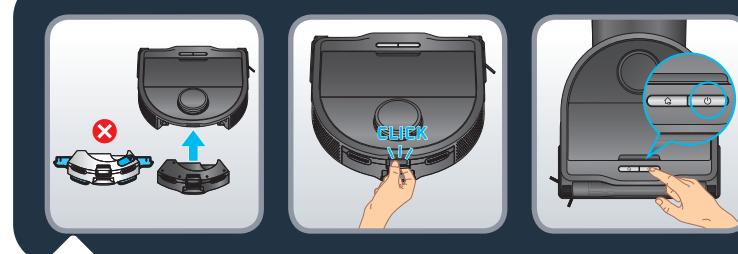
To use the robot without the mopping function ("vacuum only" mode), install the "vacuum only" module at the back of the robot. The module is correctly installed when you hear a « click » sound. Press the « Start » button or use the app to start cleaning. Keep the "vacuum only" module installed in the robot when you don't use the mopping function. The "vacuum only" module is equipped with charging contacts to allow the robot to dock to the station and to charge its battery.
