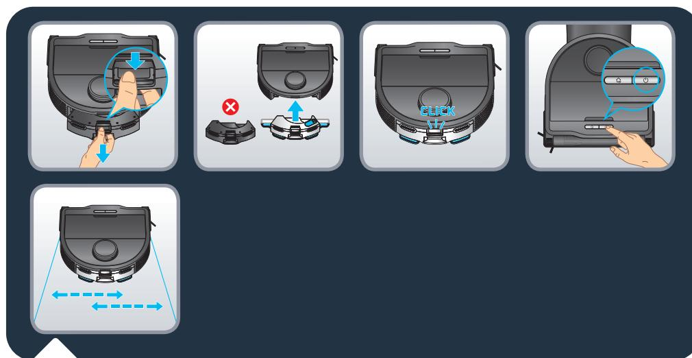
Unclip the "vacuum only" module by pressing the latch and pull to remove the "vacuum only" module. Take the water tank and clip it at the back of the robot. The water tank is correctly installed when you hear a « click » sound. Press the « Start » button or use the app to start cleaning. The vibrating mop bracket will be automatically activated with a left-to-right motion.
