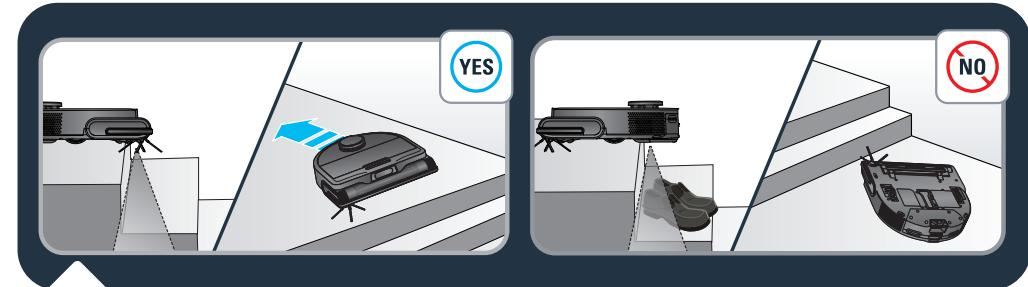
The robot has anti-drop sensors to detect stairs. The robot will change direction when detecting them. For optimum anti-drop sensors efficiency, remove any item (ex: shoe) from the stairs. When using the robot in a raised area, place a physical barrier at the edge of a drop to prevent accidental falls.
