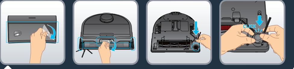
Remove all protections (protective films) on the station and on the robot. Reverse the robot, install the side brush by gently clipping it. The side brush is correctly installed when you hear a click sound.
