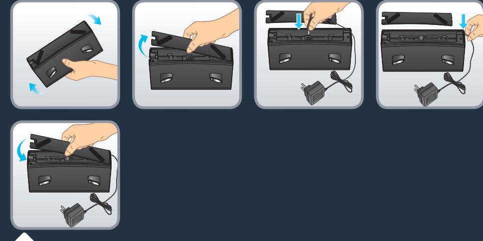
Turn the station upside down. Remove the bottom cover of the docking station and connect the adapter. Pay attention to arranging adapter connection wire to avoid being wound during sweep. Put the bottom cover back.
