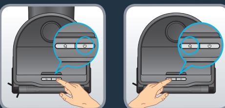
Press the button « Start » to start automatic cleaning. The robot will scan the area. It will automatically split the room into small zones, first cleans inside the zone in a zig zag, and then cleans zone edges. The robot will clean all accessible area, zone by zone. Press the button « Start » at any time to pause cleaning and press it again to resume cleaning. If the robot is on standby, press the button « Start » once to wake up the robot and a second time to start cleaning.
