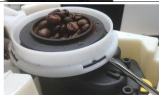
Unscrew the 2 screw of the grinder
