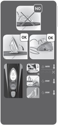
Do not place the soleplate of the iron directly on the ironing board. Use the heel or the base.
