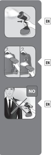
Press the steam button with the steam brush facing away from you holding it in a vertical position.
