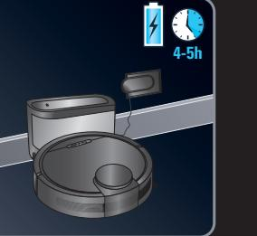
**EN** Wait 4-5 hours for the robot to be fully charged. When the white indicator is normally set on, the robot is fully charged.
