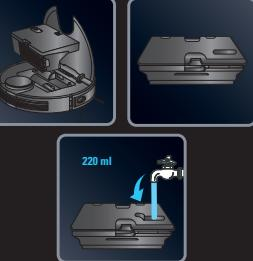
**EN** Open the robot cover, press the release button and remove the dust box and the water tank.
