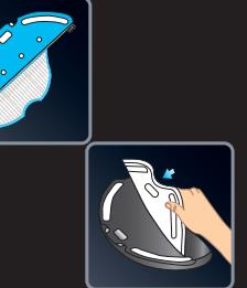
**EN** Slide the mop into the slot and put it correctly on the mop holder.
