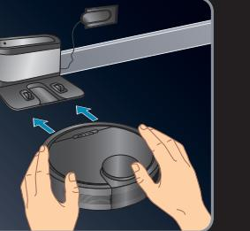
**EN** Place the robot on the docking station and align it to the charging terminal. When the robot is correctly plugged, the docking station light will switch off.
