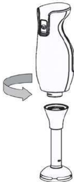
Figure 1. Mounting the metal foot of the rod blender
