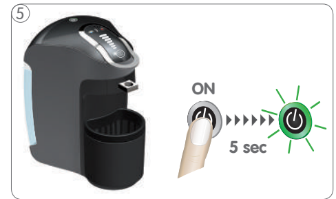
Press and hold power button for at least 5 seconds. Power button starts blinking green and machine enters the descaling mode.
