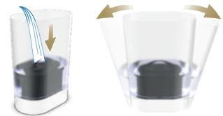
③ Install new water filter. Fill water tank half way with fresh drinking water. Then tilt the water tank back and forth to remove air bubbles from the water filter.
