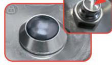
Press on the internal part of the springloaded safety valve to check that it is not clogged.
