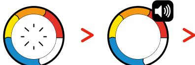
en - Flashing white coloured light: preheating in progress.
