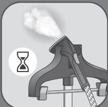
**EN** Let the appliance run until water tank is emptied completely.
