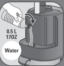
**EN** Fill .5L(Liter) of water in the appliance water tank.
