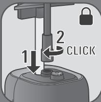
**EN** Insert the steam hose , and lock it, by screwing until hearing a "click".
