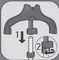
**EN** Fully insert the hanger / holder vertically on top of the pole and lock it.
