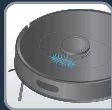
X-plorer Serie 75 S and S+: When the white indicator on the top of the robot is flashing slowly, the device is waiting for connection. When the white indicator is normally set on, the device is connected.
