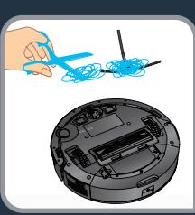
X-ploer Serie 75 S and S+: To clean the side brush, remove it by unclipping it. Remove the hair wound before replacing it back on the robot. Clean the side brush once a month.
