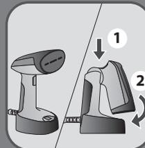
**EN** For storage purposes or to place in the travel pouch, it is possible to fold the appliance. Always press the head unlocking button before folding the head.
