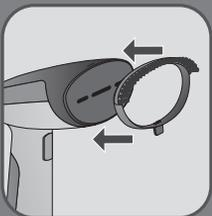
**EN** The fabric brush opens the weaves of the fabrics for better steam penetration. Before removing or attaching the steam brush, unplug your appliance and allow it to cool down, for one hour.
