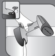
**EN** Empty the water tank completely and then close the water inlet cap.
