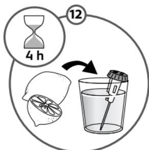
**8. EN Anti-calc valve cleaning** (once a month) / **ES Válvula de limpieza antical**
