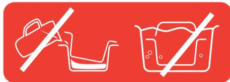
In the event of accidental immersion of the appliance or if water is spilt directly on the heating element when the pot is not in position, take the appliance to an Approved Service Centre.
