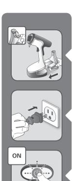
Return the water tank to its place on the appliance. Make sure the water tank is fully set in place.
