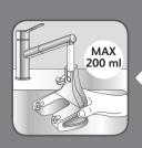
Fill the water tank with a maximum of 200 ml of untreated tap water.  $\,$
