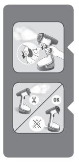
Put the steam trigger in the locked position. place the product on a flat, stable, horizontal and heat resistant surface.
