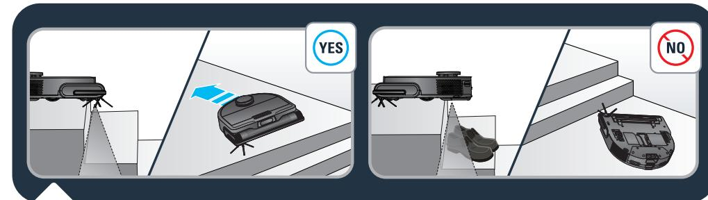
The robot has anti-drop sensors to detect stairs. The robot will change direction when detecting them. For optimum anti-drop sensors efficiency, remove any item (ex: shoe) from the stairs. When using the robot in a raised area, place a physical barrier at the edge of a drop to prevent accidental falls.
