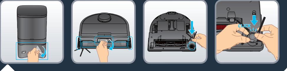
Remove all protections (protective films) on the station and on the robot. Reverse the robot, install the side brush by gently clipping it. The side brush is correctly installed when you hear a click sound.
