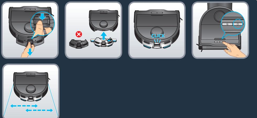
Unclip the "vacuum only" module by pressing the latch and pull to remove the "vacuum only" module. Take the water tank and clip it at the back of the robot. The water tank is correctly installed when you hear a « click » sound. Press the « Start » button or use the app to start cleaning. The vibrating mop bracket will be automatically activated with a left-to-right motion.
