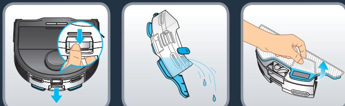
At the end of the cleaning session, unclip the water tank by pressing the latch and pull to remove the water tank. Empty the water tank of the remaining water. Remove the dirty mop cloth.
