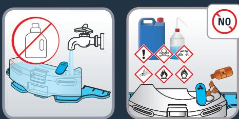
Open the stopper of the water tank and fill it with clean water until the water tank is full. Do not use hot water. Warning: Do not add cleaning agents in the water tank.
