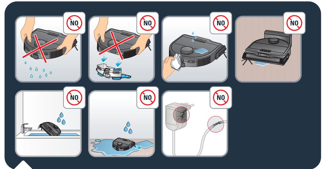
Do not shake the robot. Do not try to disassemble the vibrating mop bracket from the water tank. Do not put water or any wet cloth on the robot. Do not charge the robot when the ground is flooded. Do not submerge the robot in water. Do not use the robot on wet surfaces or surfaces with standing water.
