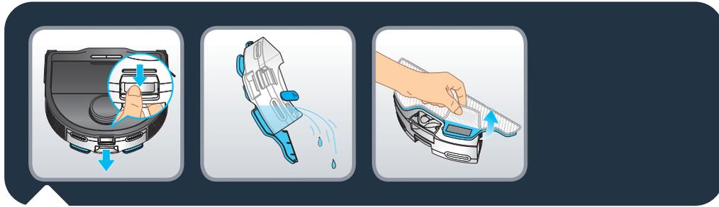
At the end of the cleaning session, unclip the water tank by pressing the latch and pull to remove the water tank. Empty the water tank of the remaining water. Remove the dirty mop cloth.
