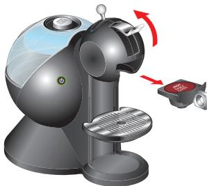
Then lift the locking handle and remove the capsule holder.
