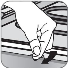
The inner glass must be lifted partly from below for a better grip. Slide the glass towards the back of the oven to release it from the notches which hold it in place.
