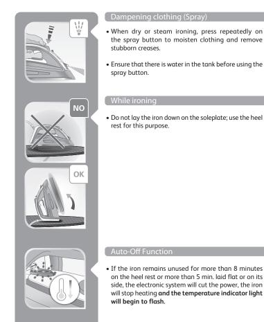
• To restart the iron, move it gently until the indicator stops flashing.
