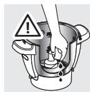
Take care with the knives of the Ultrablade knife (F1) and the kneading & grinding blade (F4) when you are cleaning them and when you empty the bowl, they are extremely sharp. Be careful if a hot liquid is poured into the food processor because it could be ejected from the appliance due to it suddenly boiling.
