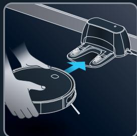
**EN** Position your robot on its docking station until the button is flashing red.
