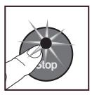
Press the stop button at any time to stop the toasting cycle.
