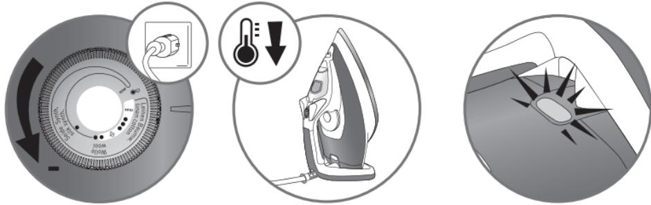
**GB** It is normal for the indicator light to switch on and off during ironing.
