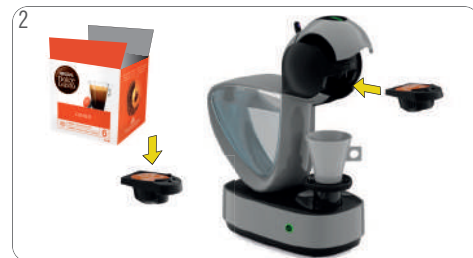
2 Clean the interior of the head. Insert a new capsule in the capsule holder and insert it back into machine.
