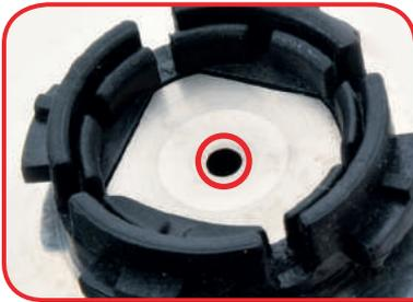
Before reinstalling the ball, check that the pipe is not blocked by blowing into it, from the opposite side to the picture above.
