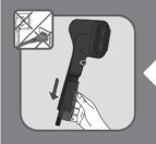
Remove the pad\* before operation. Remove the water tank by sliding it down.
