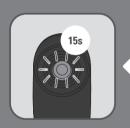
Wait at least 15 seconds before pressing the steam button. The light indicator switches off when it is ready.
