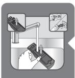
Fill the water tank with 100% water and repeat the operation until the water tank is completely empty in order to rinse the appliance.
